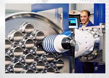
FEST-SPAN manufactures according to customer specifications or own calculations products such as heat exchanger plates for the power station industry, the chemical and petro-chemical industry, the food industry, for fertilizer production, oil coolers and other cooling systems, as well as valve trays and filter plates.
